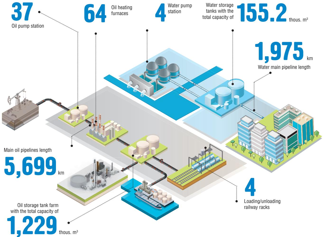
Oil transportation and transshipment through main pipelines are provided by 37 oil pumping stations, 64 oil heating furnaces and the oil storage tank farm with the total capacity of 1,229 thous. cub. m. Oil transshipment to other types of transportation means is provided by 4 loading/unloading railway racks, appropriate oil loading equipment installed on berths of the onshore oil loading terminal at Aktau Sea Port.
